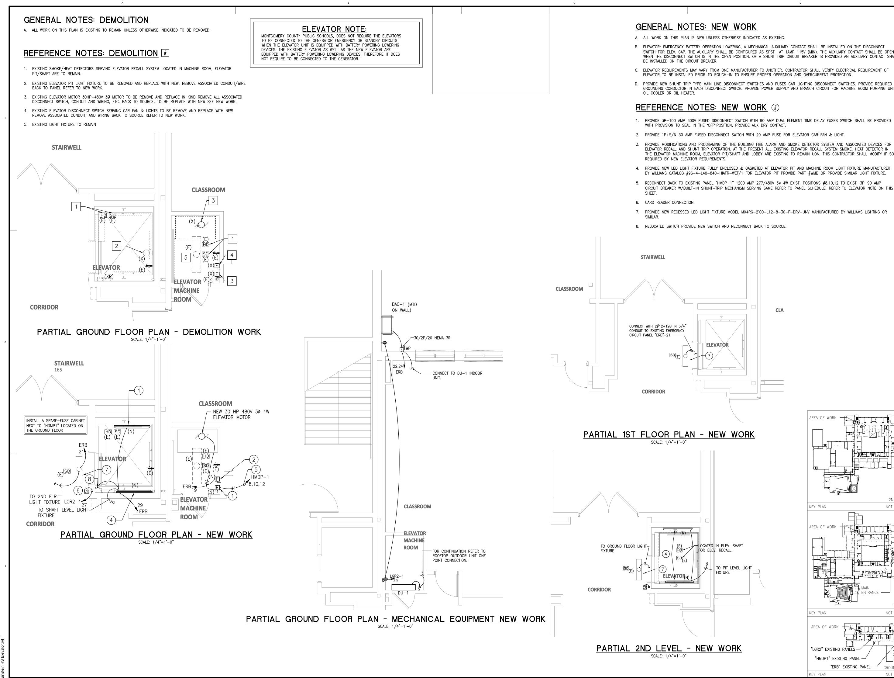
B. ELEVATOR: EMERGENCY BATTERY OPERATION LOWERING, A MECHANICAL AUXILIARY CONTACT SHALL BE INSTALLED ON THE DISCONNECT SWITCH FOR ELEV. CAP. THE AUXILIARY SHALL BE CONFIGURED AS SPST AT 1AMP 115V (MIN). THE AUXILIARY CONTACT SHALL BE OPEN WHEN THE DISCONNECT SWITCH IS IN THE OPEN POSITION. OF A SHUNT TRIP CIRCUIT BREAKER IS PROVIDED AN AUXILIARY CONTACT SHALL
